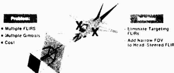
Figure 12. Consolidating the pilotage and targeting functions in a single FLIR eliminated the multiple FLIR cost problem.
