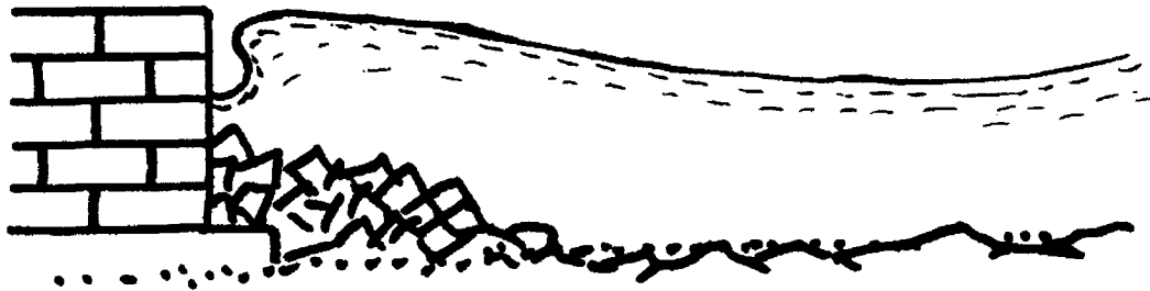
Figure 1 Sketch of a typical wave impact situation
