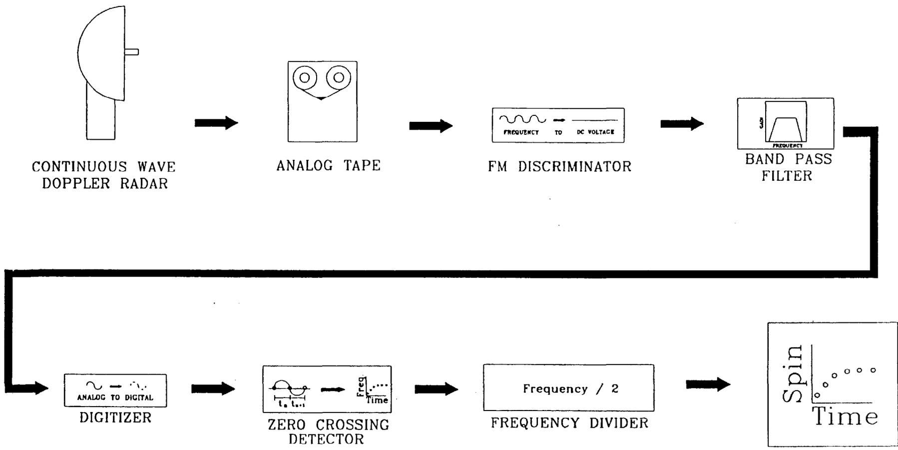
Figure 12. Equipment Used to Reduce the Doppler Data.
