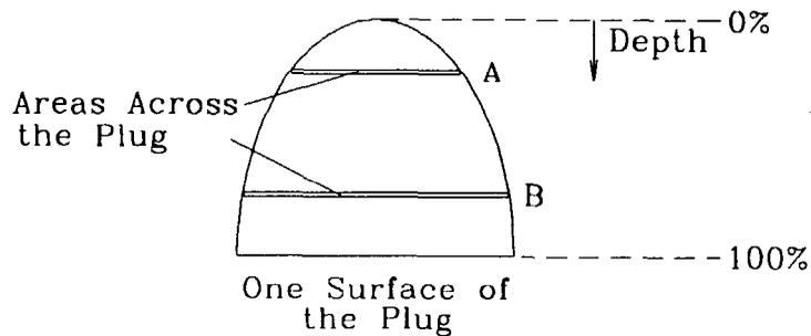
The area across the plug at A is less than that at B.
