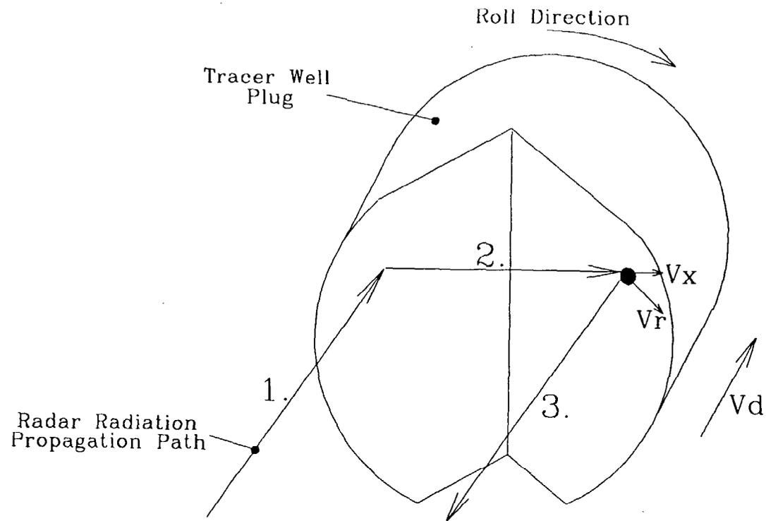
1. Radiation hits plug and Doppler shift,  $f_{d1}$ , due to  $V_d$  is created.
