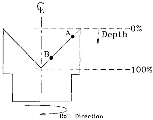
The tangential velocity at point A is greater than that at point B.
