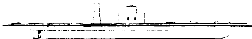
Fig. 9. Union Passiac Class monitor ( Weehawken , Patapsco , Nantucket , Nahant , Montauk , Catskill , and Passiac involved in April 7, 1863 attack on Fort Sumter). Armament: one 11-inch and one 15-inch Dahlgren smoothbores.
