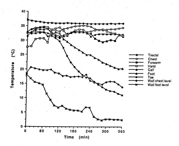
Figure 2. Temporal evolution of the skin temperature at 6 body sites, and the rectal temperature of a subject sleeping in a Cocoon-4 sleeping shelter during a 6 hours' night in the climatic chamber at -35°C, 10% relative humidity, and 2.5 km·h<sup>-1</sup> wind velocity. The temperature of the wall at two locations inside the shelter are also presented.
