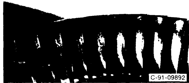
Figure 10.—Test side face gear after 30 milion pinion cycles at 100 percent torque.
