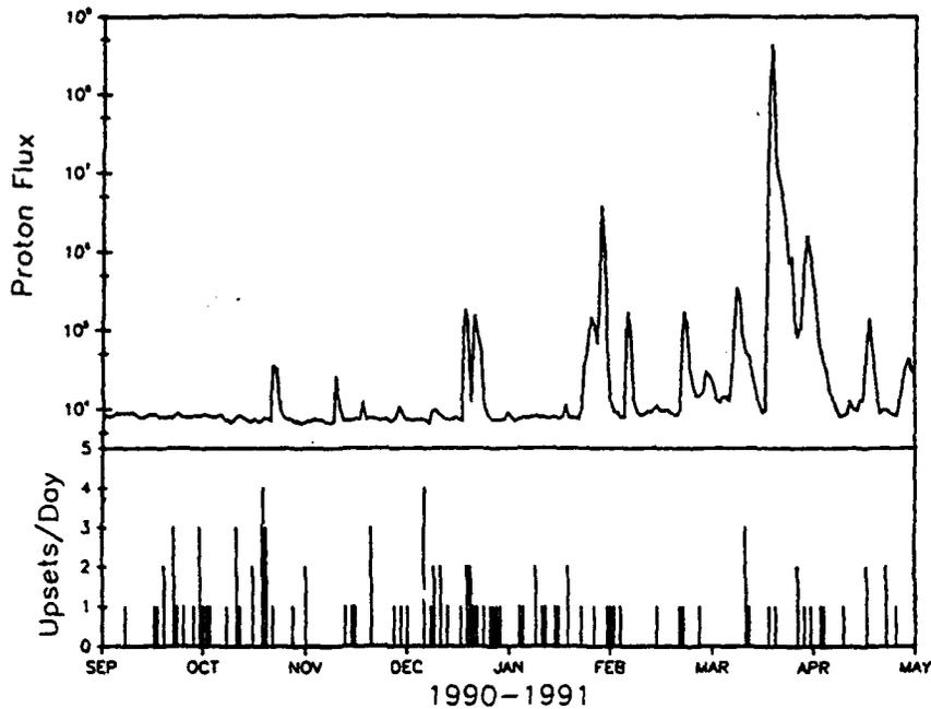
Figure 9. SEU Upset Rate vs Solar Proton Flux
