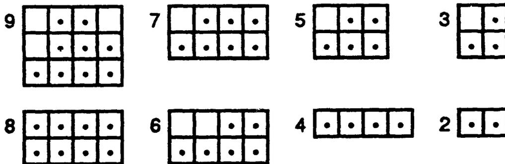
Figure 7. Typical Multiple-Bit Error Clusters (Each box represents a single location)
