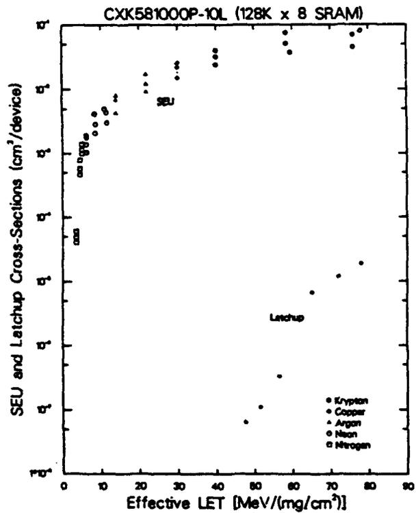
Figure 3. SEU and Latchup Results for CXK581000P
