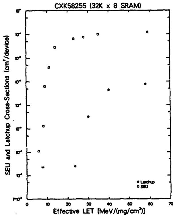
Figure 4. SEU and Latchup Results for CXK58255P
