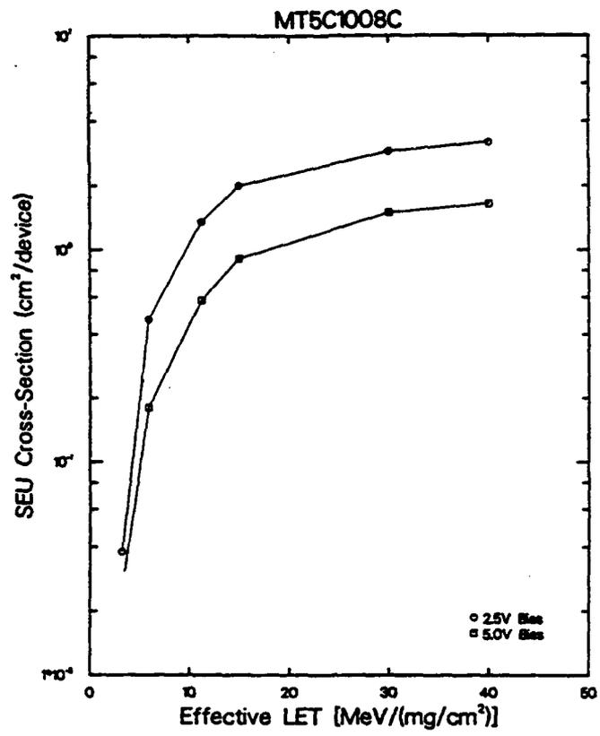
Figure 8. SEU Cross Section at 2.5 and 5.0 Volts Bias
