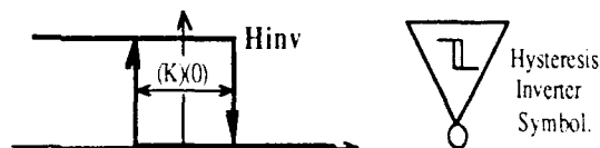
Figure 13 : Hysteresis inversion : a fundamental non-linearity.
