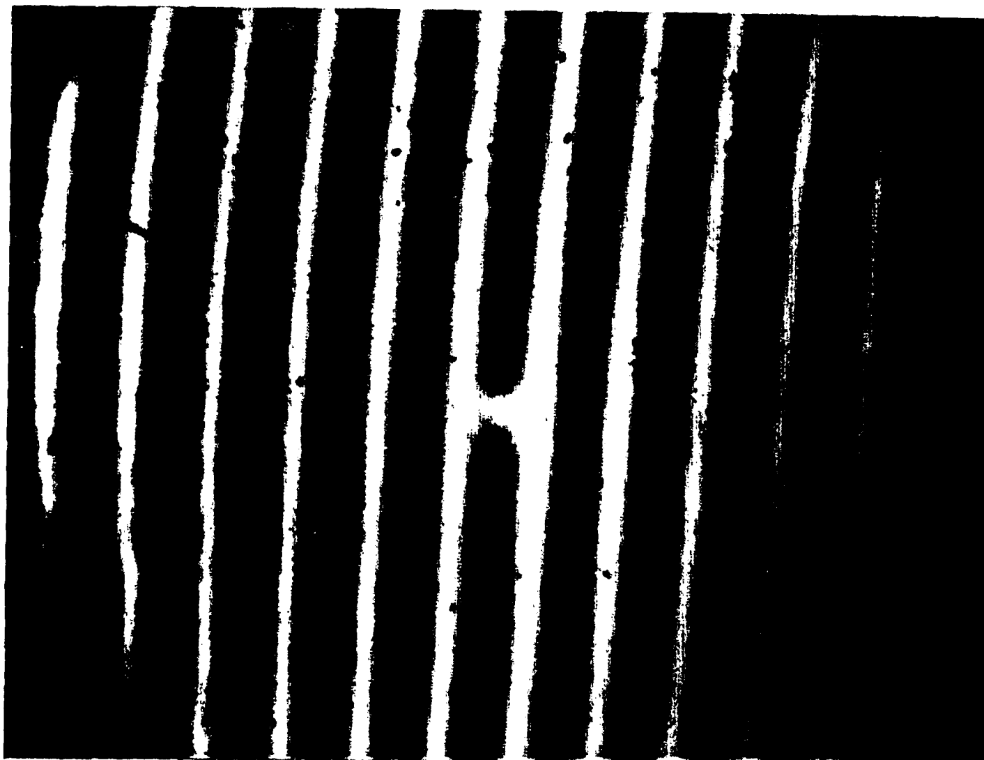
SUBAPERTURE 2: GRATING IN-FOCUS, MIRROR STRONGLY MISALIGNED
