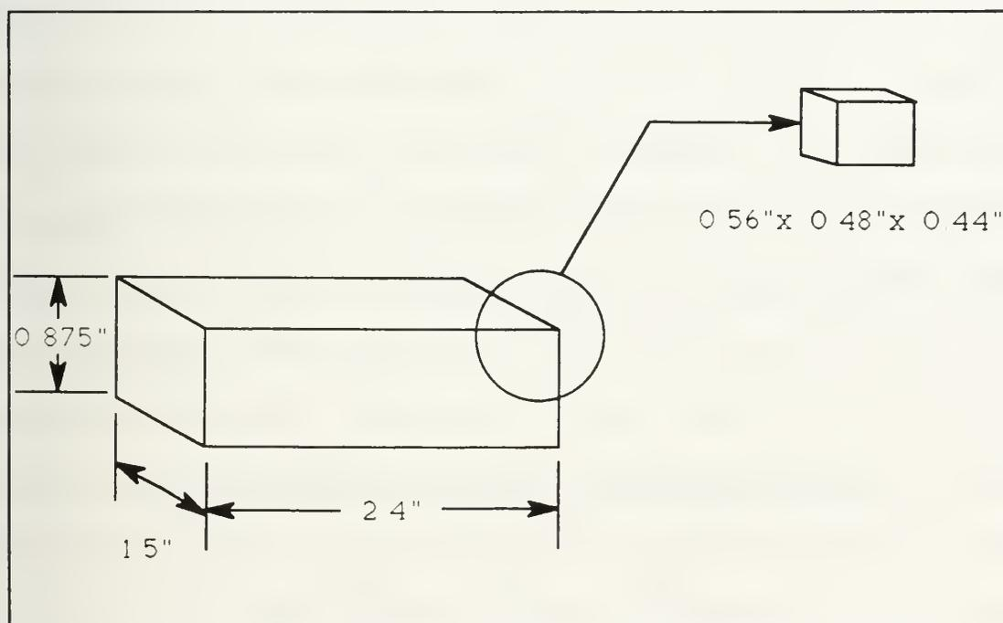
Figure 3.1 Billet and coupon geometries used for testing.
