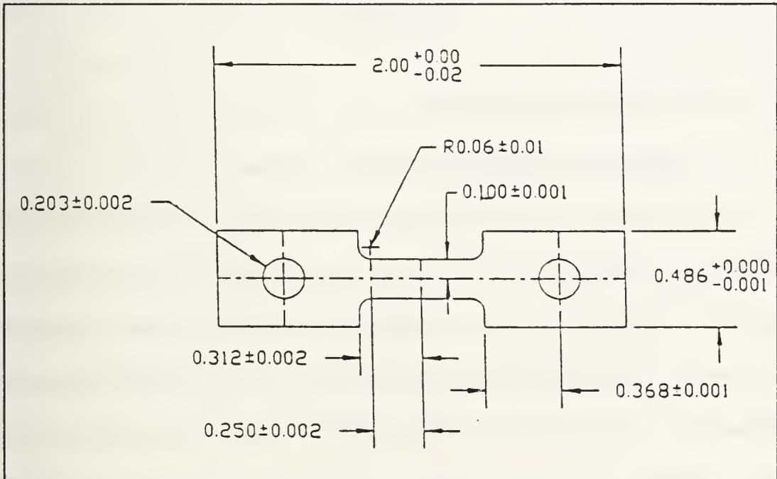
Figure 3.6 Tensile Test Specimen Drawing.
