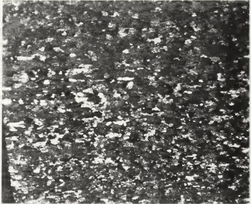
Figure 4.11 (c) 30 min., 400°C post TMP anneal.
