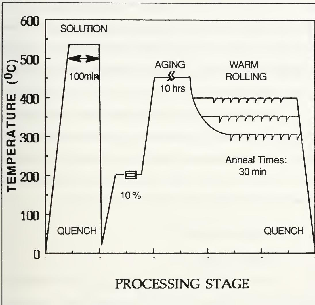
Figure 3.5 TMP Schematic Diagram.
