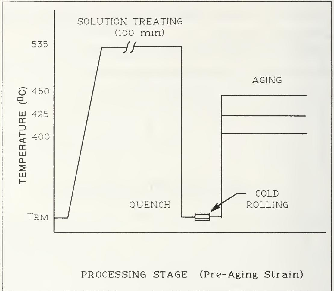
Figure 3.3 Overaging Process Diagram (Initial Cold Work).
