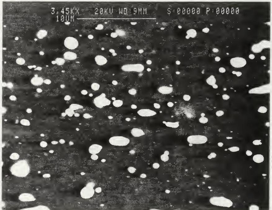
**Figure 4.10** Backscattered SEM micrograph showing the Al-Cu 2519 following TMP process 400°C roll. (a) no post-roll anneal; (b) 30 min. post-roll anneal.
