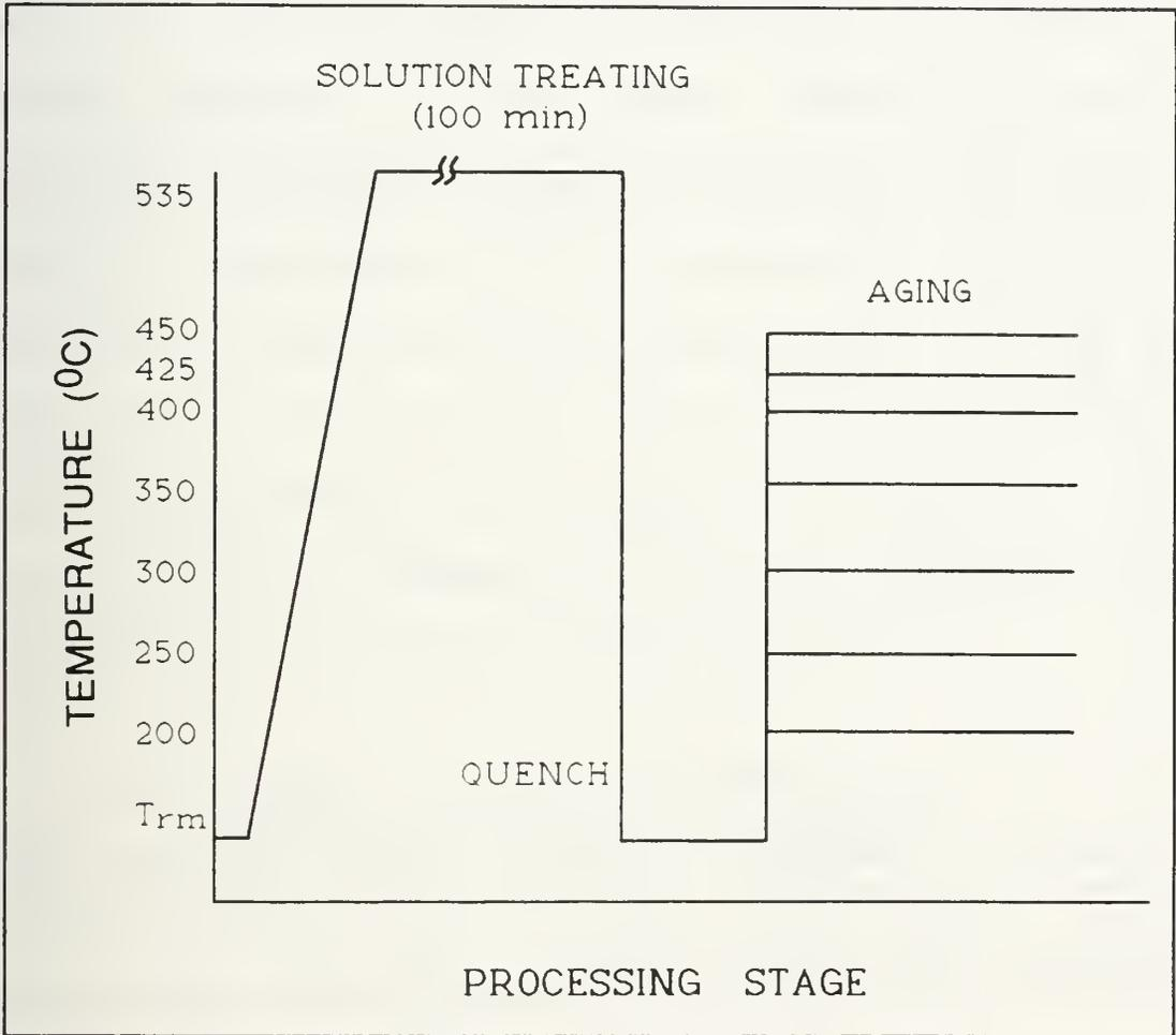
Figure 3.2 Overaging Process Diagram.
