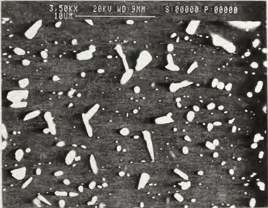
Figure 4.7 Backscattered SEM micrograph showing the Al-Cu 2519 alloy after aging for 50 hours. (a) 400°C; (b) 450°C.
