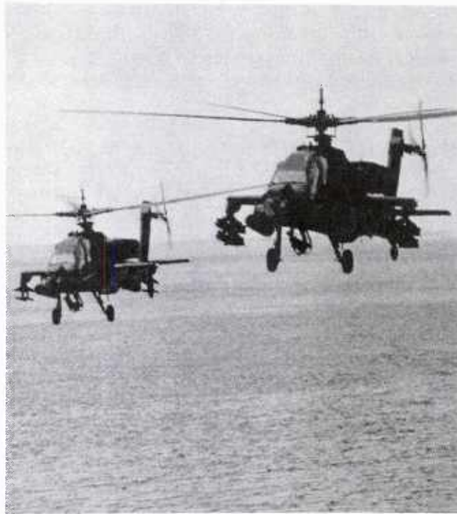
Figure VIII-18 AH-64 Apache Helicopters Returning From a Combat Mission Note: Aircraft on right has Hellfire missiles, aircraft on left has expended its ordnance
