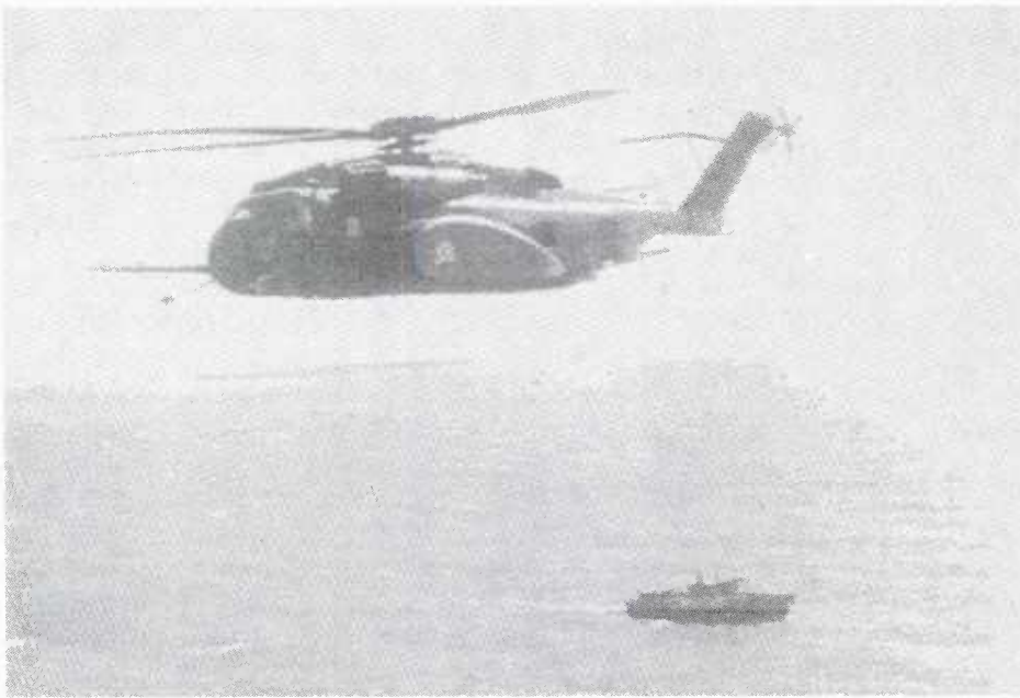
Figure VII-16 A Navy MH-53E AMCM Helicopter Conducts MCM Operations near a Royal Navy Hunt Class Mine Hunter in the Persian Gulf
