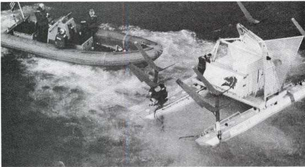
Figure VII-17 Members of Helicopter Mine Countermeasures Squadron 14 (HM 14) Prepare a Mark 105 Hydrofoil Minesweeping Sled for MCM Operations
