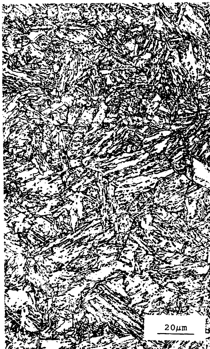
Figure 27. Light micrograph of HSLA-100 steel showing the martensitic-bainitic microstructure.
