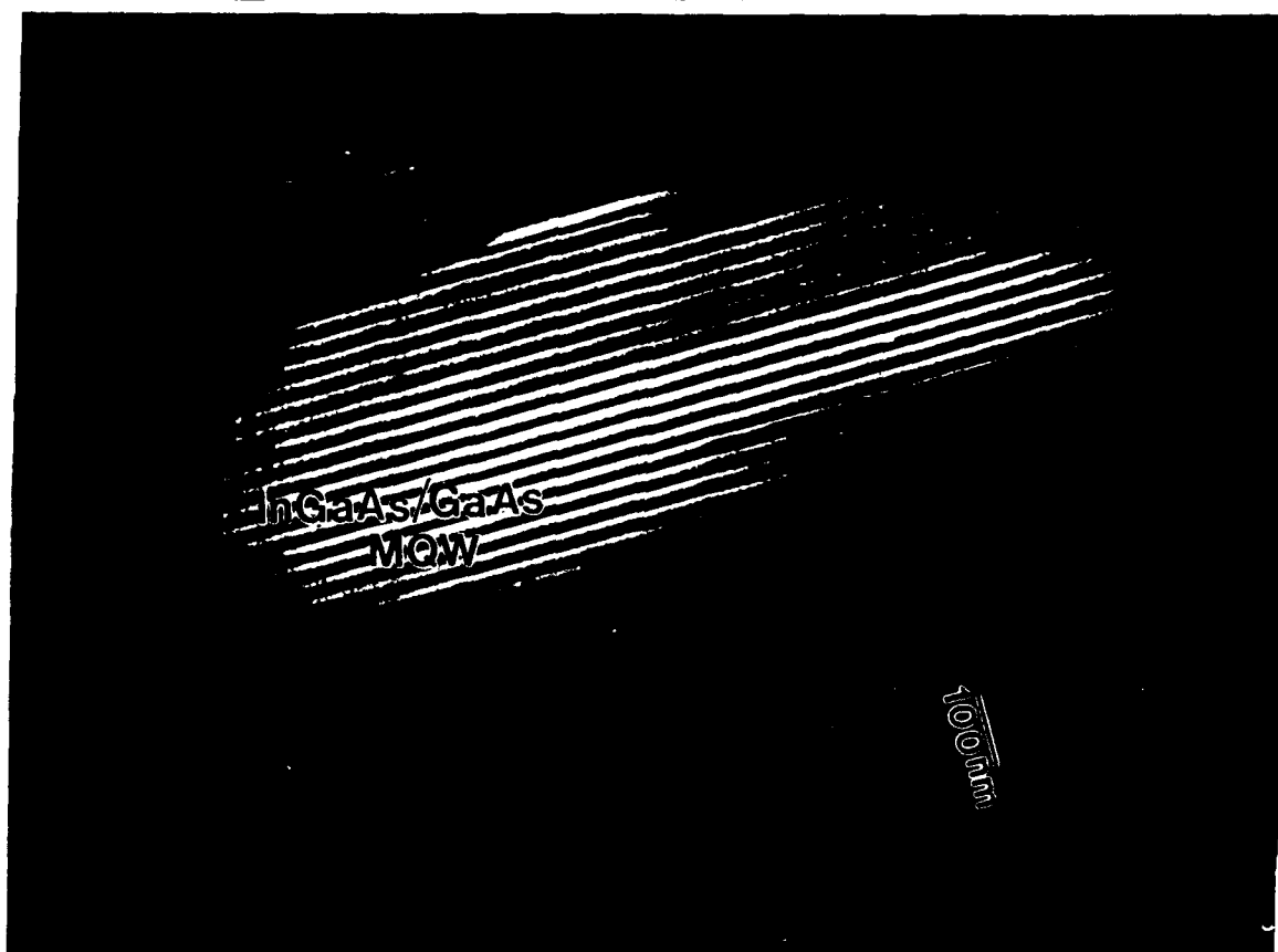
Fig. 9(b) : Shows cross sectional TEM image of the MQW in the central region on top of the prepatterned mesas.
