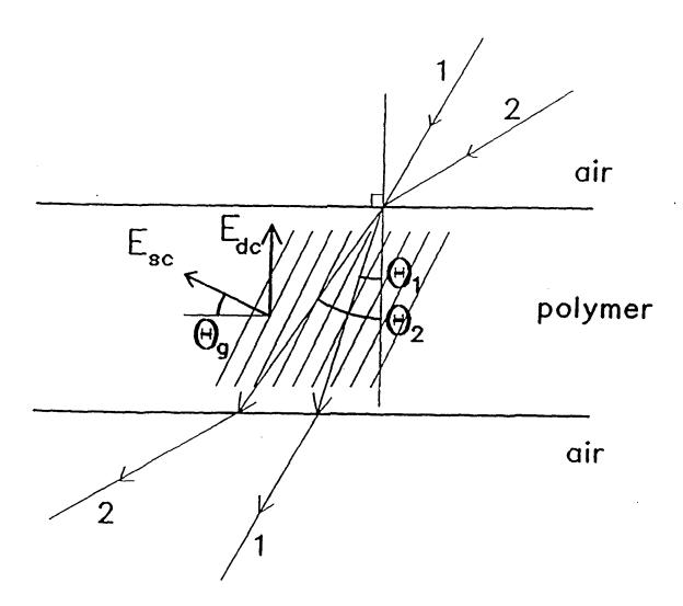
Figure 1. Geometry used for writing the grating and determining the grating phase using two-beam coupling.  $E_{dc}$  is the externally applied dc poling field, and the space charge  $E_{sc}$  is in the direction of the grating wavevector,  $K_g$ . The angles are defined in the text.
