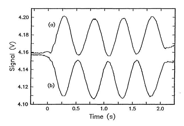
Figure 2. Transmitted intensities of beam 1 (a) and beam 2 (b) as the grating is translated. The rate of translation is 3.2  $\mu$ m/s. Motion begins at time=0 and stops at  $\approx 2.1$  s. These data have been taken in the high field regime (Eg,dc = 37 kV/cm) and the shape of the modulations indicate an index grating with 90° phase shift. Trace (b) has been offset downward by 0.02 V for clarity.
