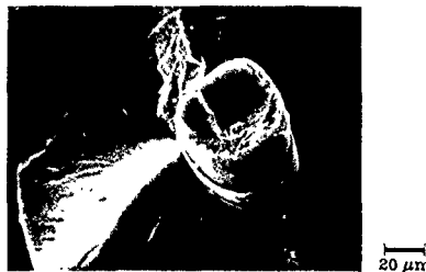
Figure 5. SEM micrograph of a typical SiC fiber fracture surface. The carbon core extends about 40 \mu\text{m} from the SiC sheath.
