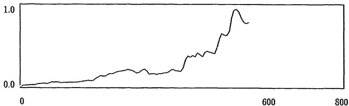
Figure 3. Iterated predictions for the Mackey-Glass equation, showing normalized mean-squared error as a function of prediction time up to 600 steps into the future.
