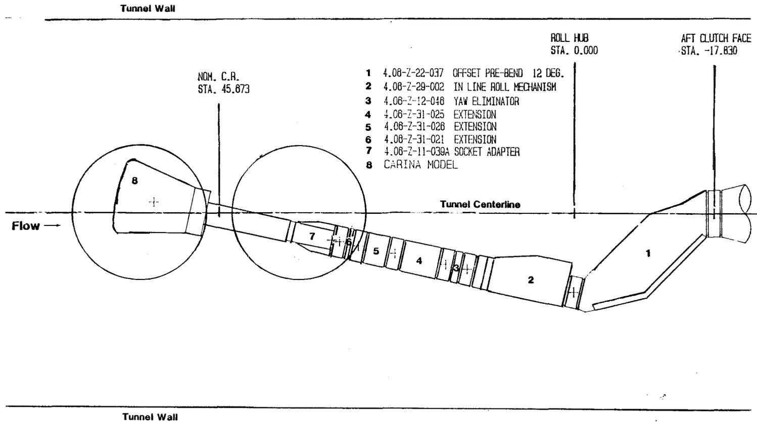
**Figure 4. Carina Installation in Tunnel B**
