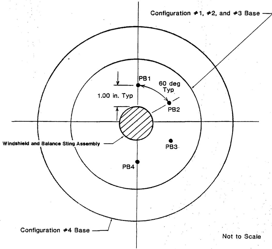
Figure 6. Carina Force Model Base Pressure Orifice Locations
