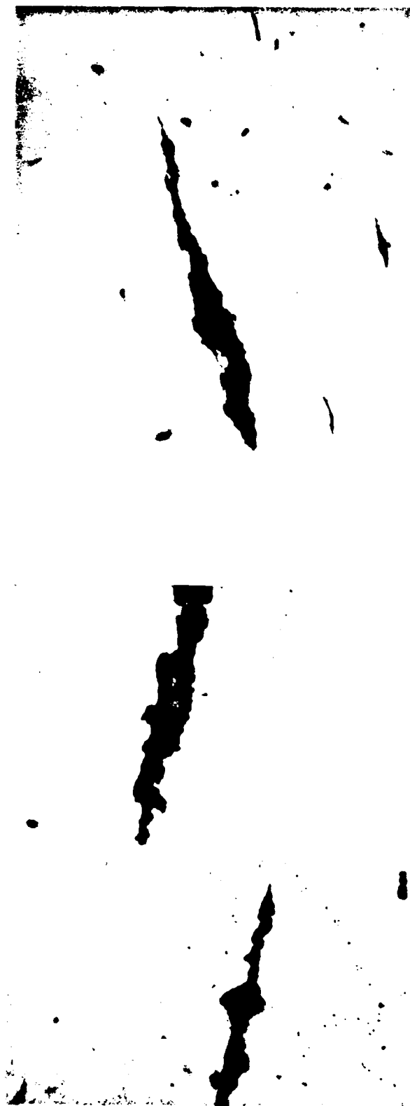
Figure 5. Oxide inclusions, as-polished (400X).
