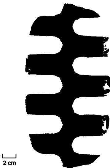
Figure B1. Tire B (NDCC 700-16LW; bias ply; 234-kPa inflation pressure; 0.0238-m 2 contact area).
