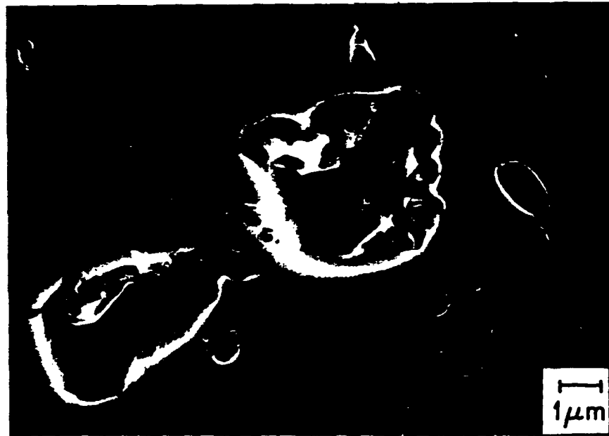
Figure 8. Pores at a polycrystalline copper-sapphire interface after being held 37 hours at 750°C under a tensile stress of 1.02 MPa.
