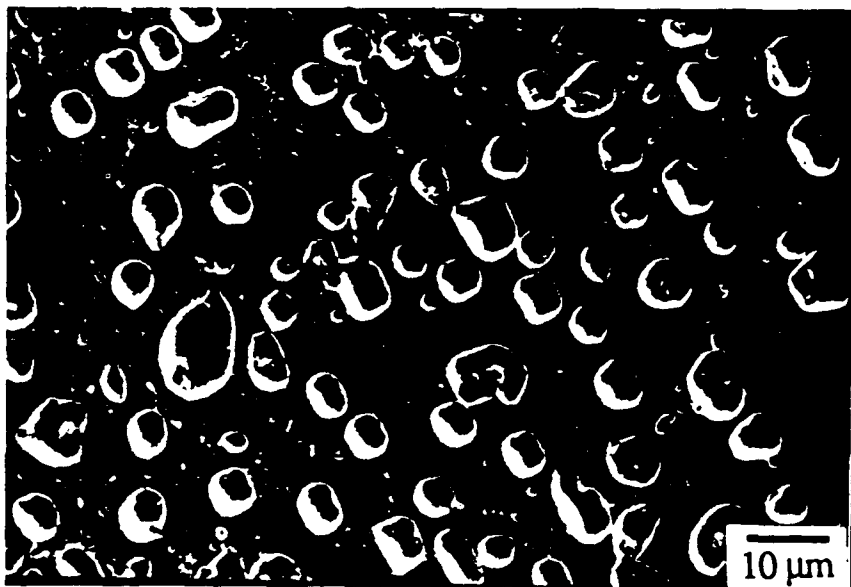
Figure 3. Pores on the copper surface of a single crystal copper-sapphire specimen held under a tensile stress of 2.64 MPa at 700°C for 48 hours. The upper photograph was taken near the edge of the specimen whereas the lower was taken closer to the middle of the same specimen.
