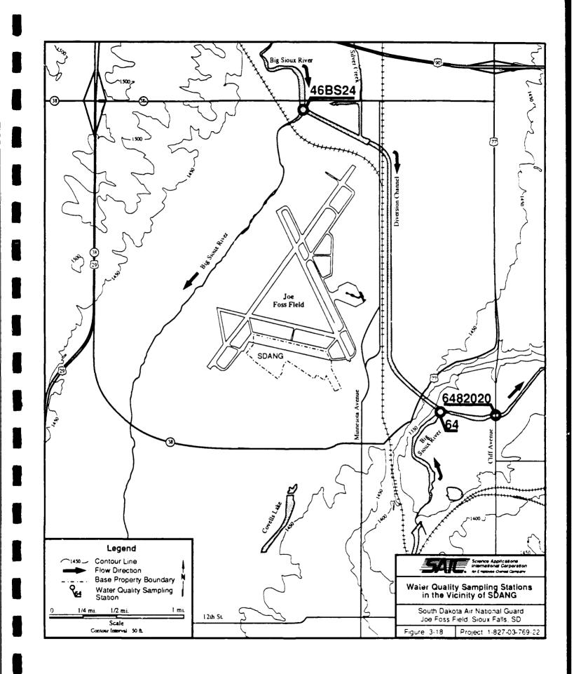
Water samples are collected from these locations on a monthly basis and analyzed for conventional, inorganic, and bacteriological pollutants (fecal coliform; ammonia; ortho- and total phosphates; conductivity; suspended solids; alkalinity; hardness; total solids; and, in May through August only, sodium, calcium, and magnesium). Testing data for 1983 through 1989 are available for each of the sites.
