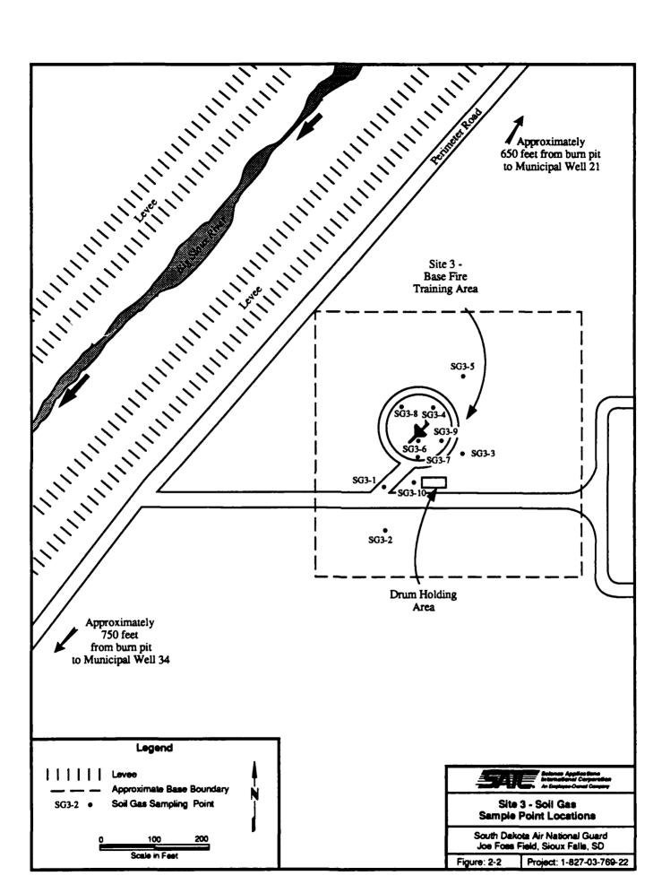
and evacuating 5 to 10 liters of gas with a vacuum pump. During this evacuation, soil gas samples were collected with a syringe by inserting the syringe needle through a silicone evacuation line and down into the steel probe. Following the collection of the sample (either soil gas or water), the probes and hollow-stem augers were extracted from the ground and the hole was backfilled with cement/bentonite grout.
