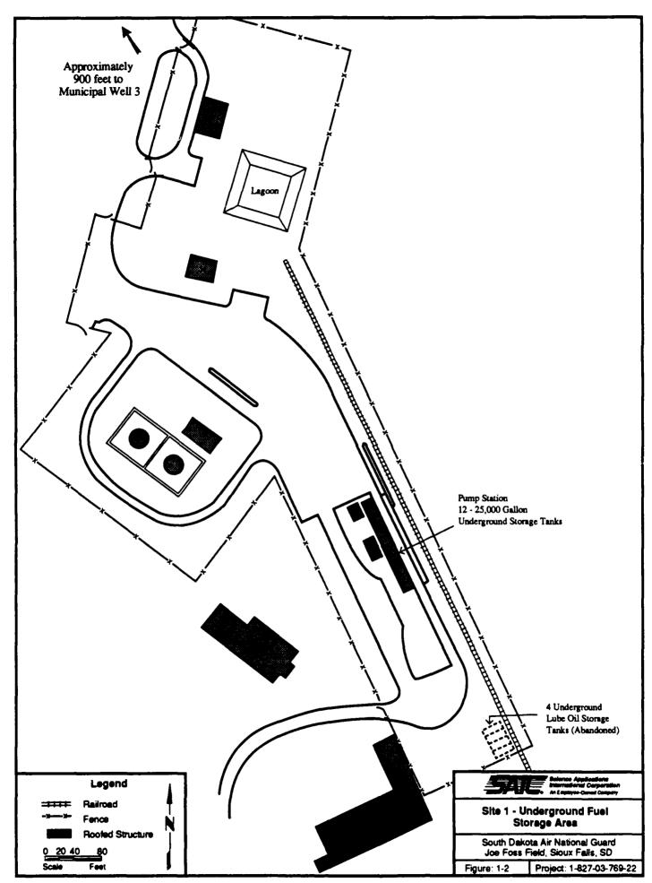
borings near the inactive tanks. According to personnel performing the borings, strong petroleum odors were noticed approximately 11 feet below land surface (BLS) and 1 to 2 feet into saturated materials in three of the four borings.
