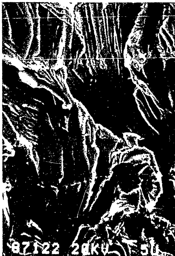
FIGURE 3—Scanning electron micrograph of the stress corrosion fracture surface of an as-received C-Mn steel specimen after failure in methanol-ammonia; (a) X450 (original magnification) and (b) X1300. Note the parallel bands on the fracture surface, which correspond to the pearlite bands in the microstructure and also the parallel sets of striations on individual cleavage facets.
