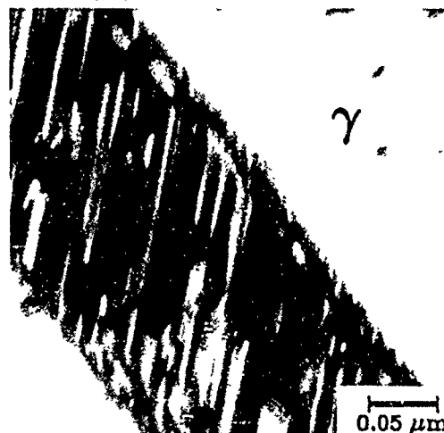
FIGURE 4—High-resolution micrograph of twinned \alpha' -martensite seen in foil prepared 1 mm under the fracture surface.
