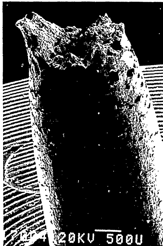
FIGURE 1—Micrograph of an as-received C-Mn steel specimen after failure by SCC in methanol-ammonia; X22.
