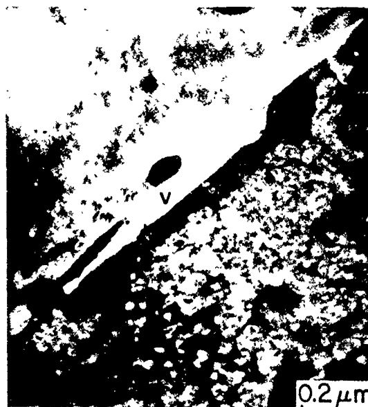
FIGURE 11—TEM micrograph of grain-boundary voiding (v) along the precipitate-free zone in a large-grained 500-ppm Pb alloy. Specimen obtained from tensile interruption test where holding at 80°C was performed prior to reloading.
