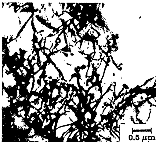
FIGURE 2—Homogeneous dislocation arrays seen 2 mm under the fracture surface.
