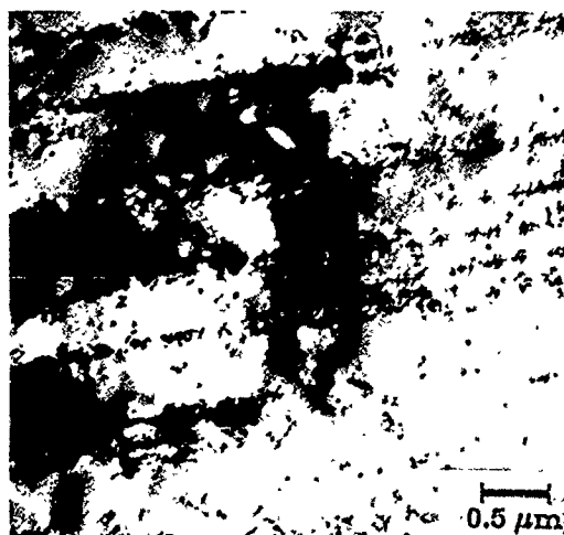
FIGURE 1—Parallel slip traces showing planar deformation at the fracture surface.
