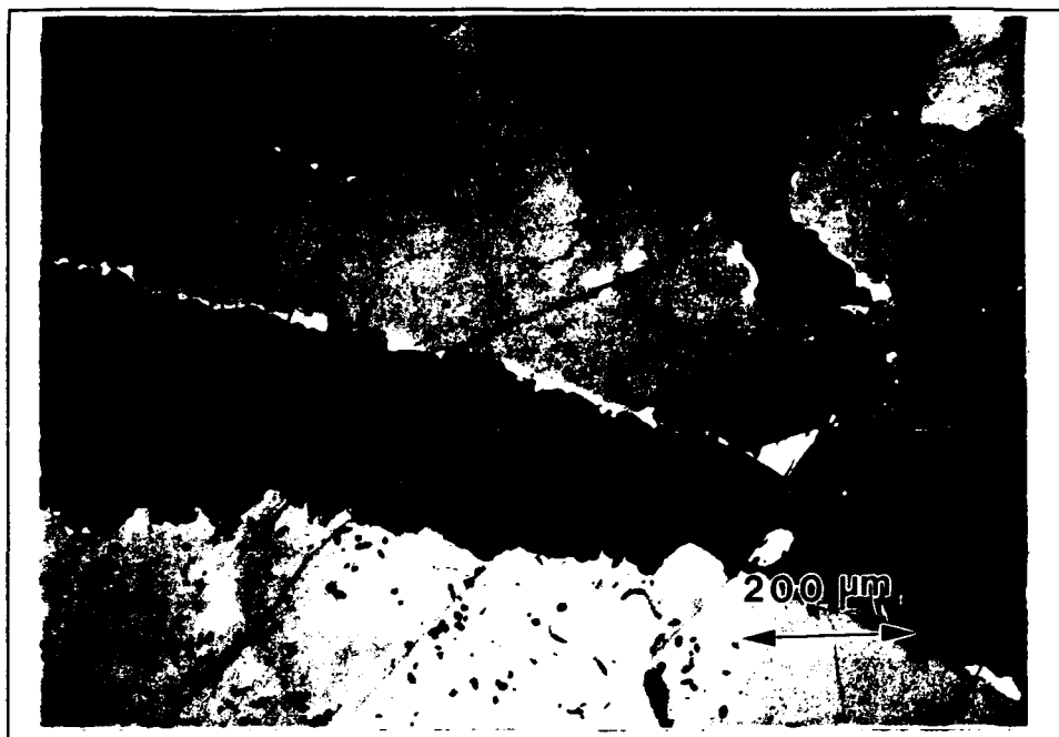
Figure 2.14 Second phase present between impinged YBCO grains in a phase pure melt-textured pellet.
