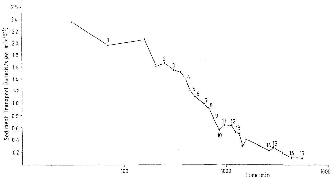
Figure 7 Decline in Sediment Transport with Time: Experiment 3
