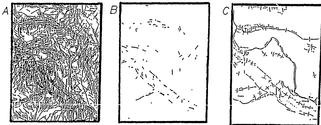
Figure 3. Synopsis diagram for the Hanford, Washington lineament study area. See Thiessen and others (1989B) for more details. A) All linear features seen on a radar mosaic, DEM image, and aeromagnetic maps. The latter includes previous interpretations by other groups as well as WSU interpreters. B) Computer generated compilation map of features within five degrees and 0.8 km of each other. To be included on this map, a single lineament had to be observed a multiple number of times on at least two of the original data bases (radar, DEM, aeromagnetic). C) Mapped faults and folds in the study area.
