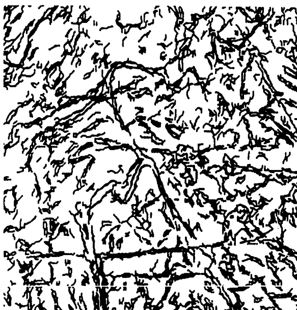
Figure 3 Edge image after Edge Following as Graph Searching has been applied to the image shown in Figure 2.
