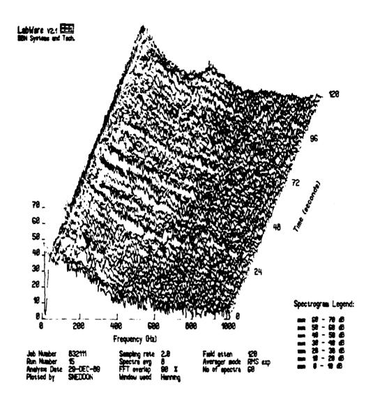
Figure 2-2: Ground Signature of an Overflight by a Stage III Aircraft at 35,000 Feet at Mach .8
