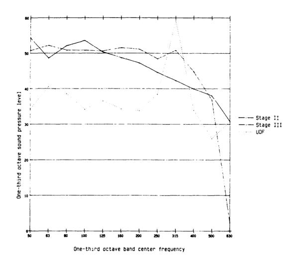
Figure 3-1: Spectral Shapes Assumed for Unducted Fan, Stage II, and Stage III Aircraft in Cruise Conditions, Normalized to 50 dBA
