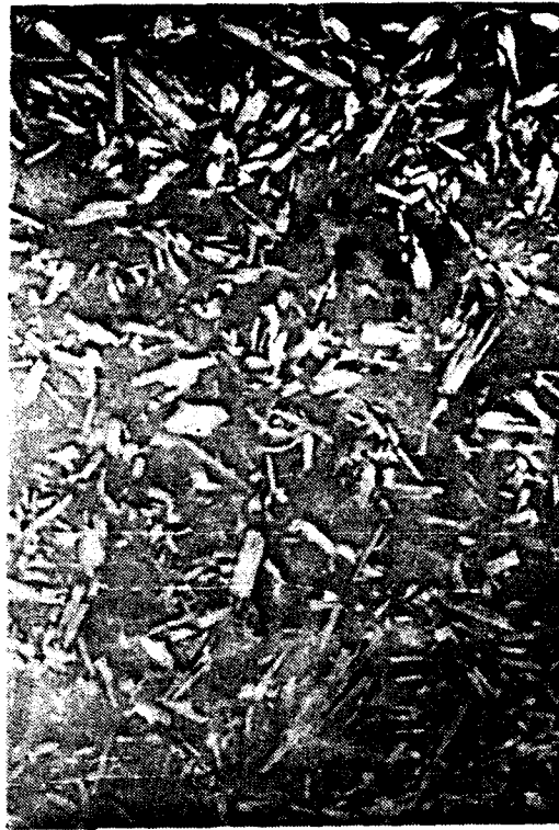
FIGURE 1. Examples of microstructure and reinforcement variants examined in the present study. a) TiB_2 -particulate (black) in a lamellar, \alpha_2 (light) + \gamma (gray) matrix, b) NbB_2 -short-fiber (white) in a lamellar, \alpha_2 + \gamma matrix, c) TiB_2 -particulate in an equiaxed, \alpha_2+\gamma matrix, and d) NbB_2 short fiber in an equiaxed, \alpha_2+\gamma matrix. Backscattered electron images at 500X.
