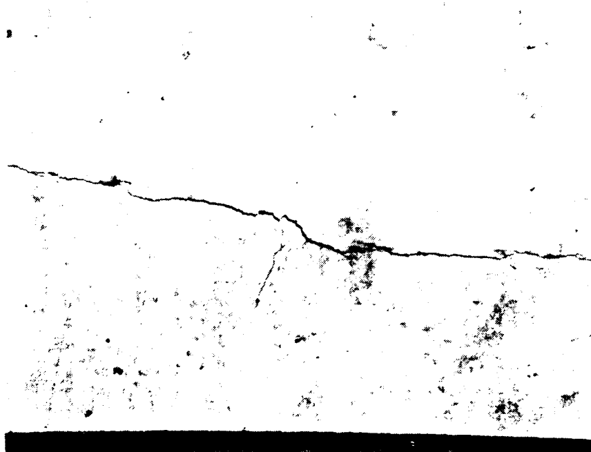
Figure 3.4.5.2-2 Front (top) and back (bottom) views (10x) of specimen D-7, which had been impacted at room temperature with an energy of 0.54 ft-lbs. Front surface shows an indentation and back surface shows a large longitudinal crack.
