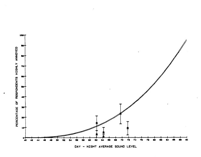
Figure 4-6: Relationship of Traffic Data from Tramway and Traffic Study to 1978 Synthesis Curve.
