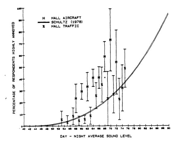
Figure 4-2: Relationship of Data from Aircraft-Traffic Comparison Study to 1978 Synthesis Curve.
