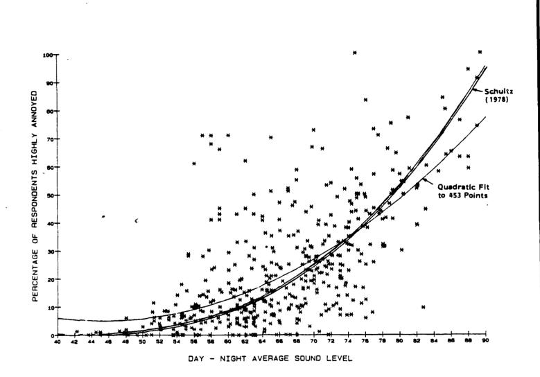
Figure 5-2: Comparison of 1978 3rd Order Polynomial Fitting Function with Quadratic Fit to 453 Data Points.
