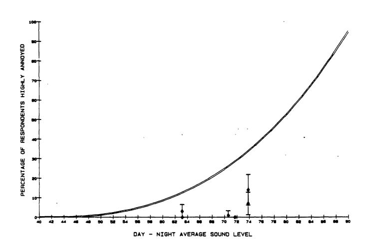
Figure 4-5: Relationship of Tramway Data from Tramway and Traffic Study to 1978 Synthesis Curve.
