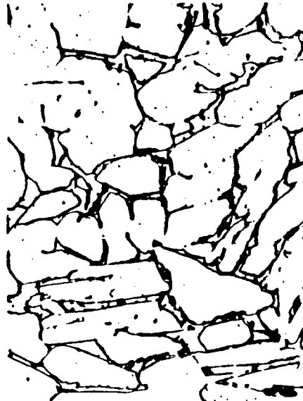
Fig 4. As in Fig 3 but at higher magnification and etched in mixed chromic and nitric acids to show more clearly the beta phase containing dark particles of a third phase. X 600
