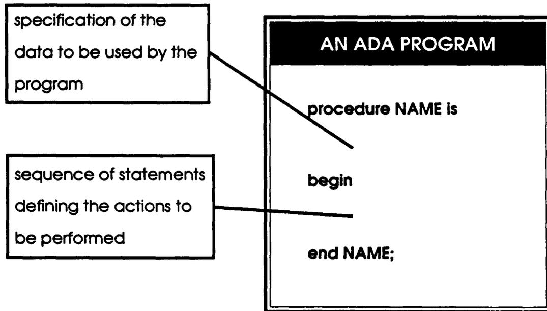
➡ **procedure** is a keyword followed by the name of the program which is chosen by the programmer. Keywords denote particular kinds of constructs. In this example, the keyword **procedure** denotes the start of a piece of program which is to be executed. Keywords are written in lower-case and programmer-defined words are written in UPPER-CASE.
