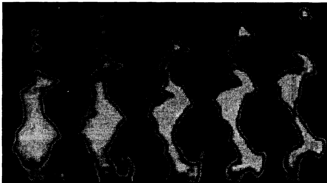
Figure 1. Consecutive images of the reactant distribution in a premixed hydrogen/air flame recorded at a rate of 48,000 frames/sec.
