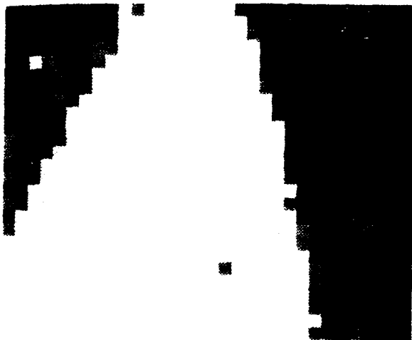
Figure 4: Road probability image. The pixels that best match typical road colors are displayed brightest.
