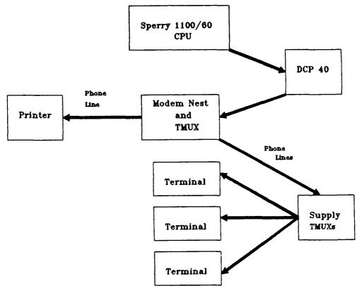
CPU - Central Processing Unit. This is the heart of the Sperry 1100/60 Computer System. All electronic manipulation of data and arithmetic functions are performed here (42).
