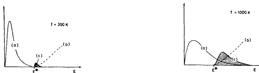
Figure 12: Variation of the reaction rate constant with temperature (a) Energy distribution function E \exp\left(-\frac{E}{RT}\right) (b) Excitation function (c) Product (a)*(b) the integral of which is proportional to k_D (from [49])
