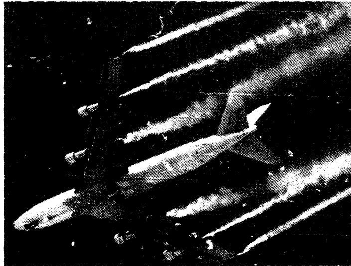
Figure 29. B-747 aircraft wake vortex patterns using corvus oil vaporizers.
