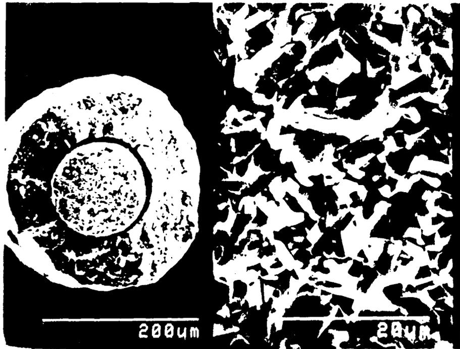
Figure 2.3.2 Silver-Palladium Clad Y-123 Wire After Continuous Sintering At 945°C in Air
