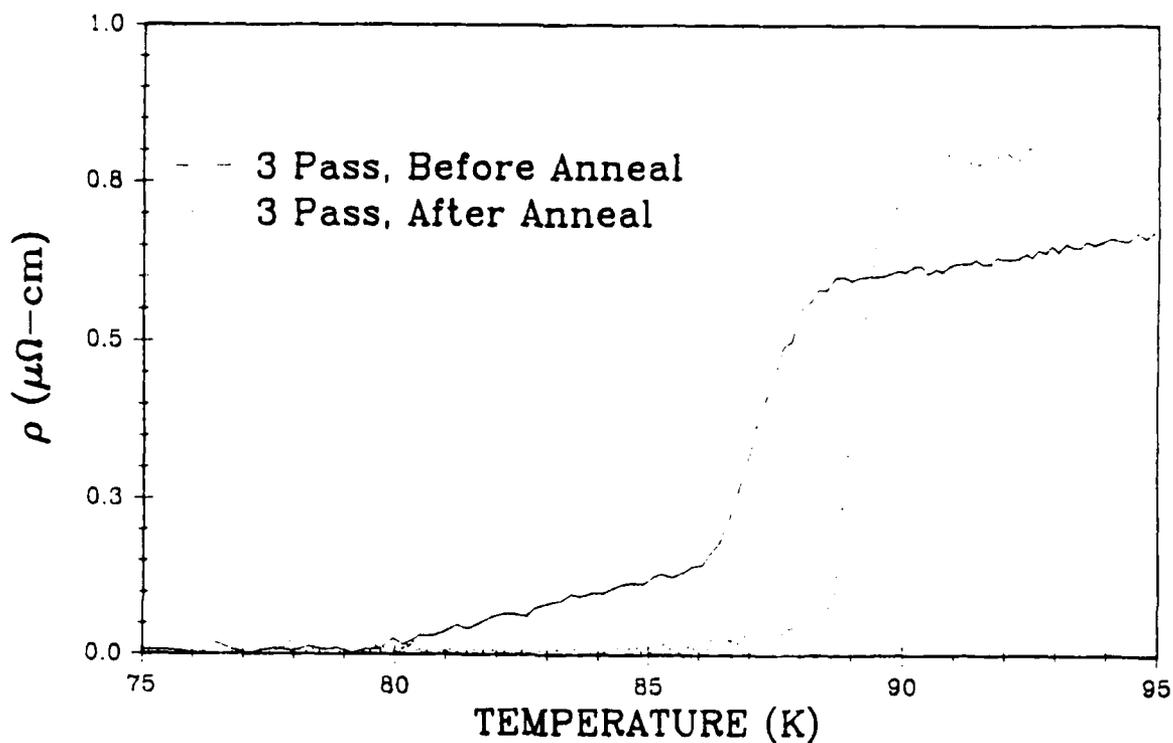
Cofired fiber, fired in air. 1<sup>st</sup> pass to 270°C, 2<sup>nd</sup> pass to 920°C, 3<sup>rd</sup> pass to 925°C.
