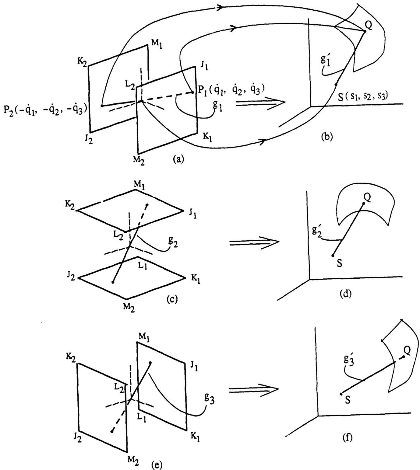
Figure 6: Quadratic mappings of a three degree-of-freedom manipulator
