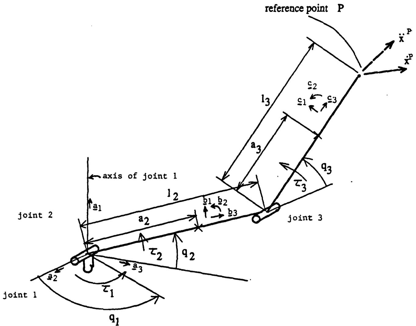
Figure 9: Schematic diagram of a three degree-of-freedom manipulator
