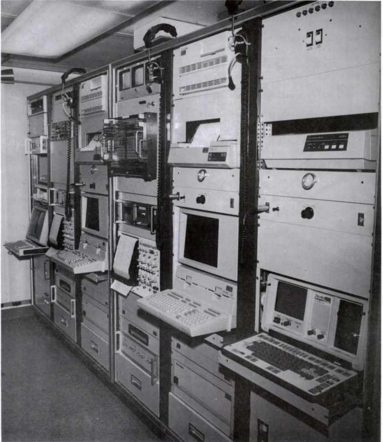
Figure 18. Photograph of the six instrumentation racks installed in the control room of the Vestibular MFL. These racks house two stand-alone data acquisition systems and related equipment required to operate and control the various biomedical tests implemented in the MFL.
