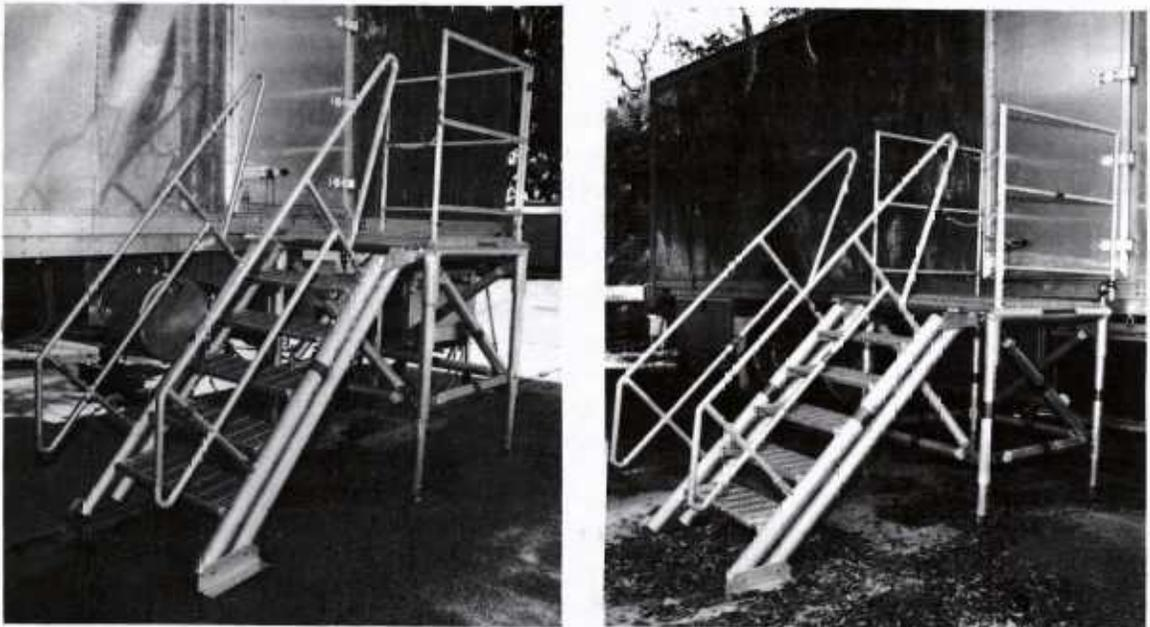
Figure 4. Curbside view of the two different modular ladder and staircase assemblies provided with each MFL. One ladder is constructed to allow access to the entrance door with stairs parallel to the trailer (left) and the other with stairs perpendicular to the trailer (right).
