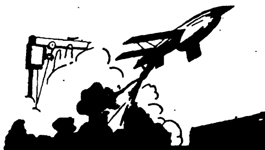
Fig. 1-8. Booster-assisted surface launch.
