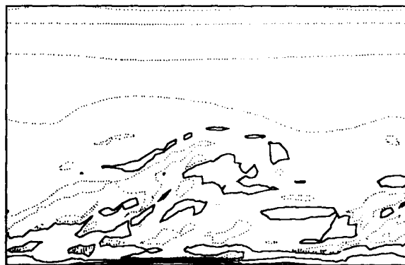
FIG. 7 Vorticity ( \omega_z ) map of an x - y section of the \pi \times \pi/8 channel described in the text. Note the laminar two-dimensional flow near the top wall, and the turbulent character near the bottom one. Vorticity isolines, \omega_z = -3, -2, -1, 0, 1, 4, 7, 10 . Dotted lines, zero or negative.
