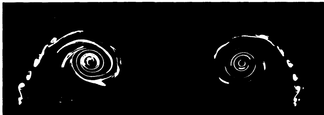
Figure 9 Laser Light Sheet View of a Forced Response Case. 70^\circ Wing at 20^\circ Incidence, 0.33m/s, 20 Hz
