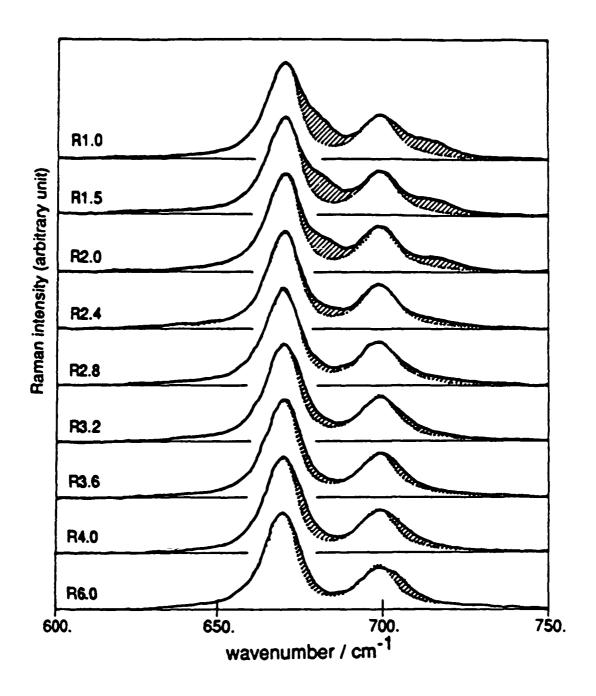
Fig. 3 The 600 to 750 cm<sup>-1</sup> region of the Raman spectra of samples with the specified values of R. Dotted lines are Raman specta of pure DMSO solvent. The shaded part is the difference between the spectrum of the sample and that of pure DMSO.
