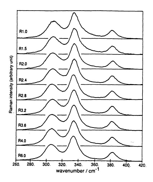
Fig. 1 The 260 to 420  ${\rm cm}^{-1}$  region of the Raman spectra of samples with the specified values of R.
