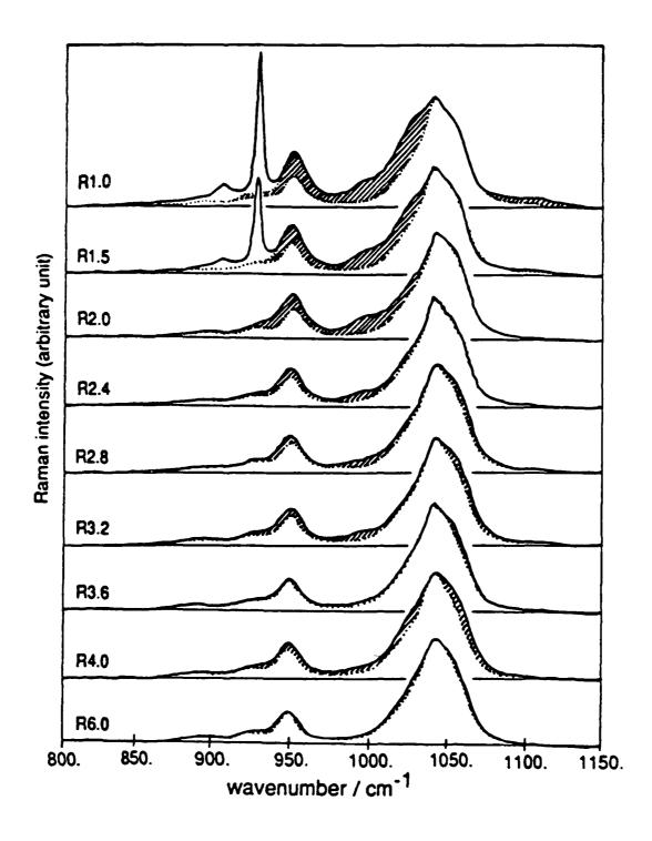
Fig. 2 The 800 to 1150 cm<sup>-1</sup> region of the Raman spectra of samples with the specified values of R. Dotted lines are Raman spectra of pure DMSO solvent. The shaded part is the difference between the spectrum of the sample and that of pure DMSO.
