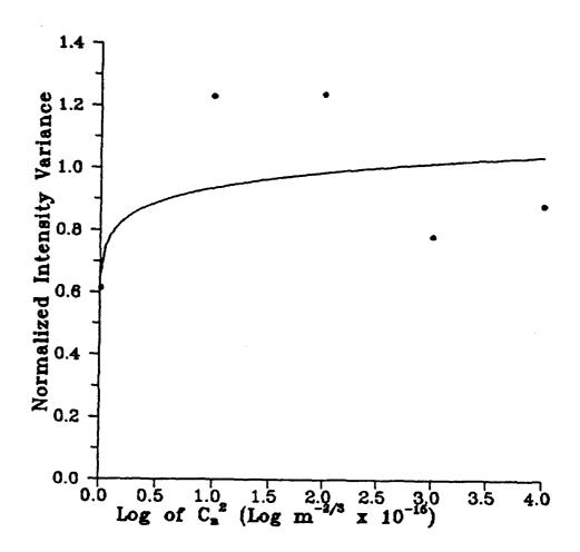
Figure 15. Intensity Variance Saturation of a 16 x 16 Subaperture.
