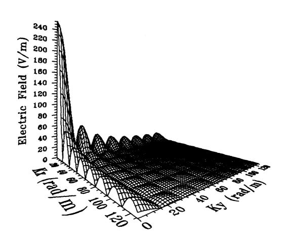
Figure 5. Three Dimensional Diffraction Pattern of a 16 x 16 Subaperture.
