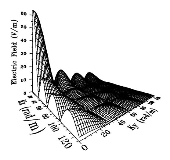
Figure 4. Three Dimensional Diffraction Pattern for an 8 x 8 Subaperture.
