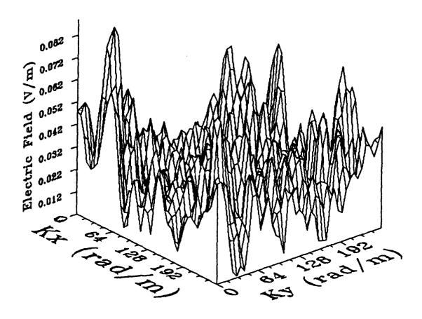
Figure 6. Perturbed Diffraction Pattern of a 16 x 16 Subaperture.
