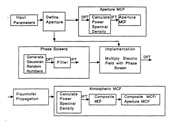
Figure 2. Conceptual Diagram of the Simulation Coding.
