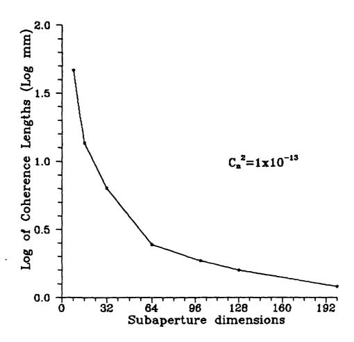
Figure 13. Subaperture Coherence Lengths for  $C_s = 1x10^{-13}$ .
