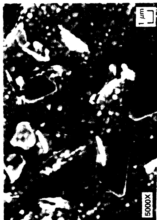
(f) Microstructure of the AC Sparkplug "TZP-110"
