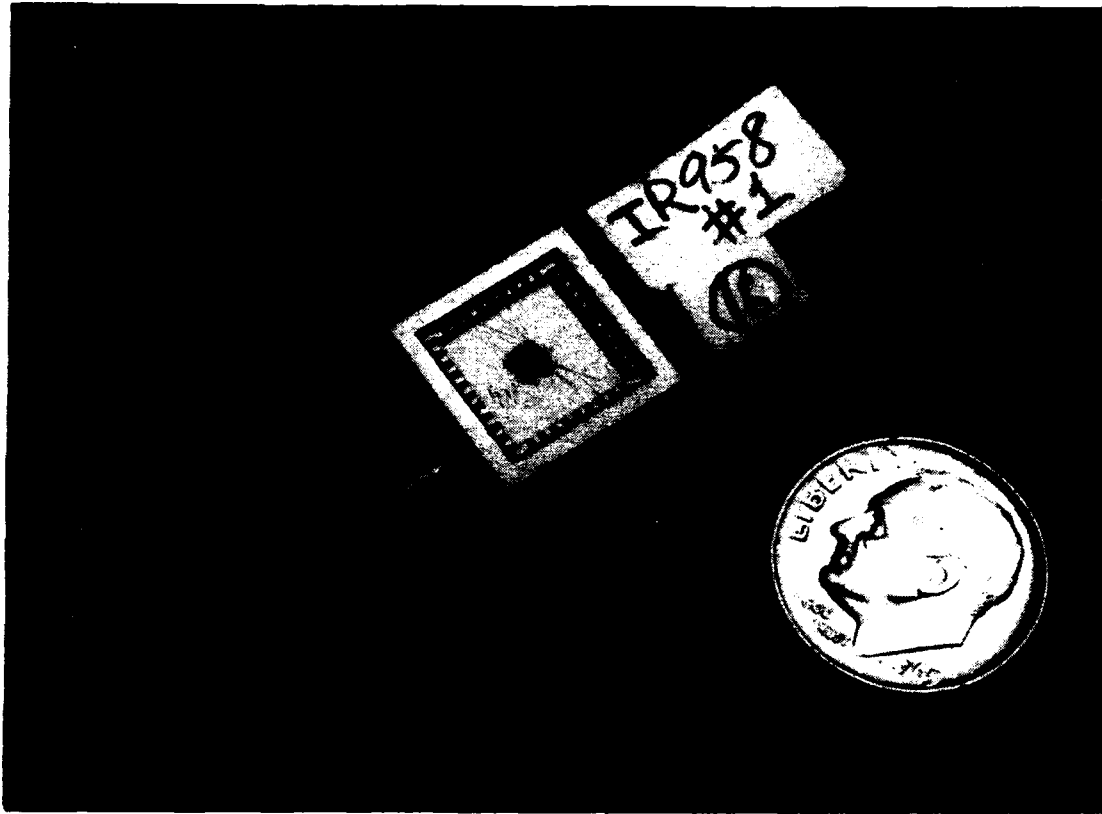
Figure 10. Picture of a SEL array mounted on a chip carrier
