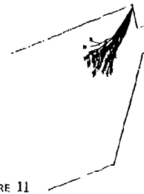
FIGURE 11 THE EFFECT OF TURBULENCE ON 45 MICRON DROPLETS.
