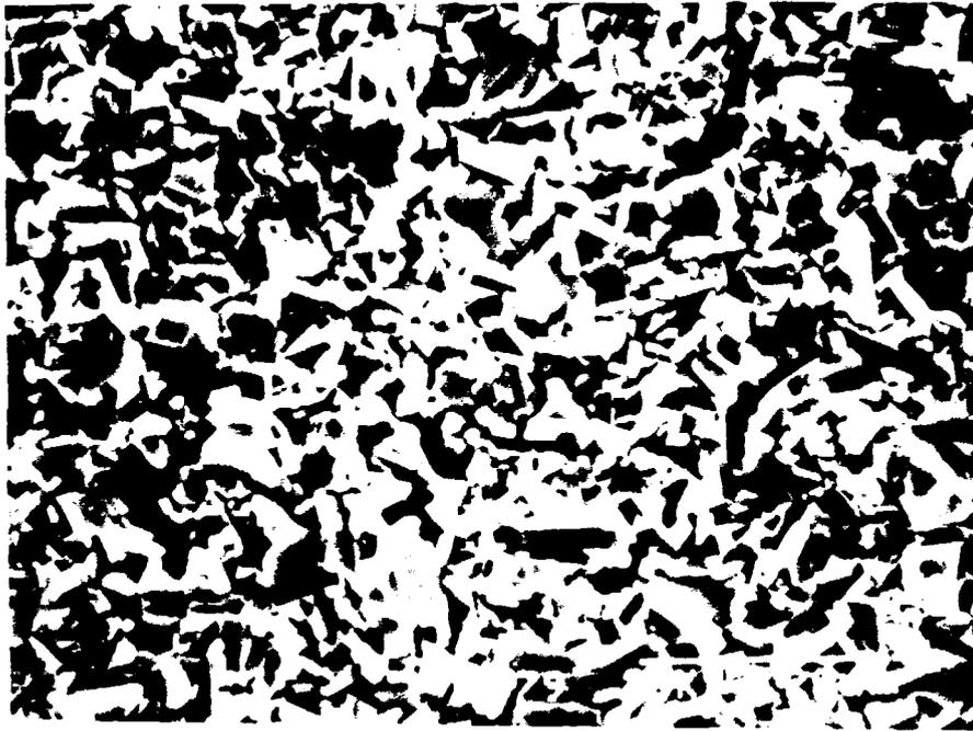
Figure 2.3.4A      Fracture Surface of  $\text{YBa}_2\text{Cu}_3\text{O}_{7-\delta}$  Filament after 2 Zone Passes at  $970^\circ\text{C}$ .
