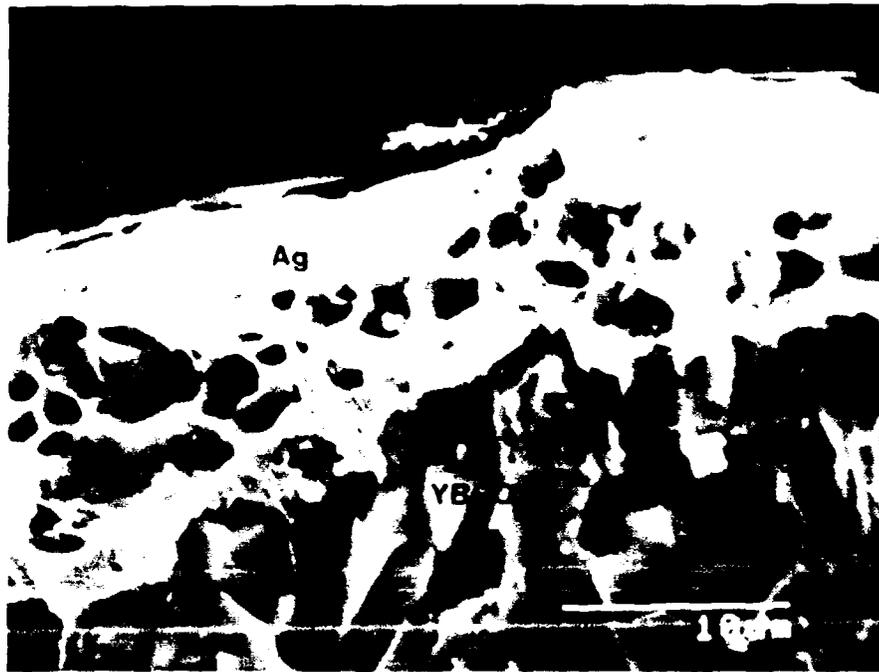
Figure 2.4.2 Fracture Surface of  $\text{YBa}_2\text{Cu}_3\text{O}_{7-\delta}$  Filament with Silver Coating Sintered at  $955^\circ\text{C}$ .
