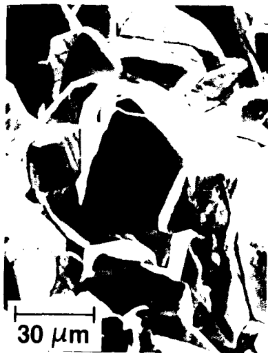
Figure 4. SEM of Chromium Electrodeposit on 304 SS. C: 2.12 \text{ mol dm}^{-3} , \eta_N: -0.6 \text{ V} , t_N: 2 \text{ s} , \eta_G: -0.05 \text{ V} , i_G: 0.025 \text{ A cm}^{-2} , l: \sim 40 \text{ μM} .
