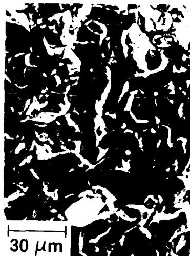
Figure 5. SEM of Chromium Electrodeposit on 304 SS. C: 1.5 \text{ mol dm}^{-3} , \eta_N: -1.0 \text{ V} , t_N: 1 \text{ s} , \eta_G: -0.09 \text{ V} , i_G: 0.07 \text{ A cm}^{-2} , l: \sim 25 \text{ μM} .
