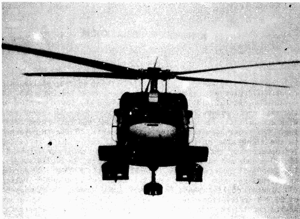
Photo 1. Front View - UH-60A Helicopter with Skis Installed
