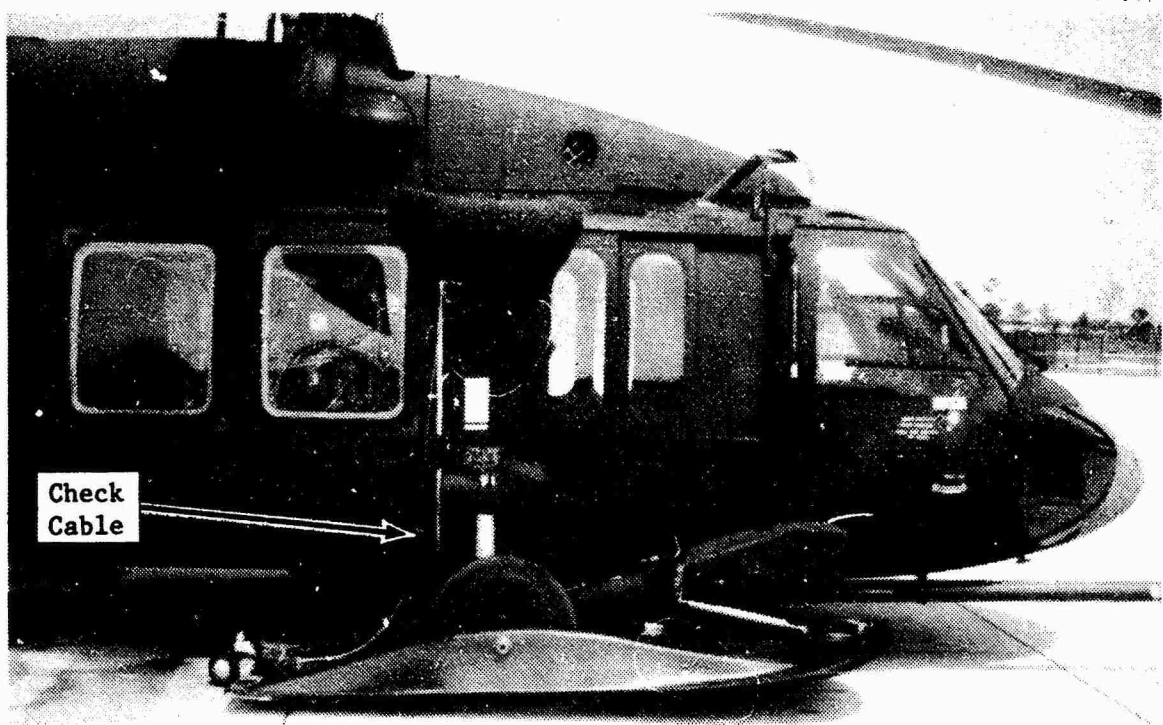
Photo 5. Right Side View - UH-60A Main Landing Gear Ski Assembly
