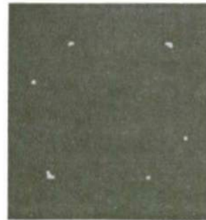
4. AFTER THRESHOLDING 3, DILATION BY b (H-Corners)
