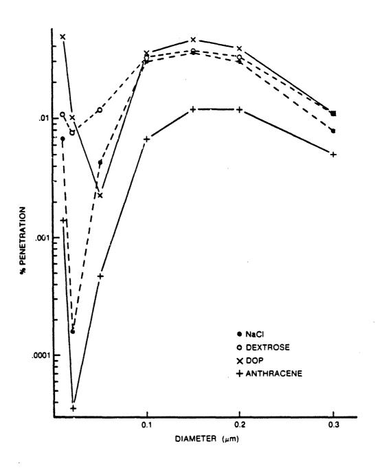
Figure 2 Detail of HV4A penetration, four cases showing extremes in behaviour.
